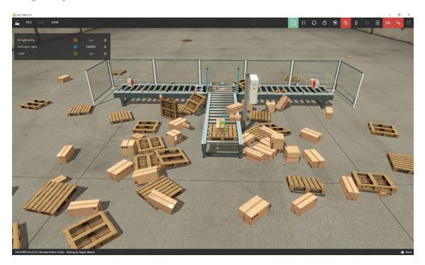
This was the result of our first testing phase of checking that Factory I/O. This test showed that Factory I/O can use PLC's to control a system and that when programmed incorrectly have a visual display that something went wrong. This was one of the reasons we chose Factory I/O for feedback and this test proved it will work.
